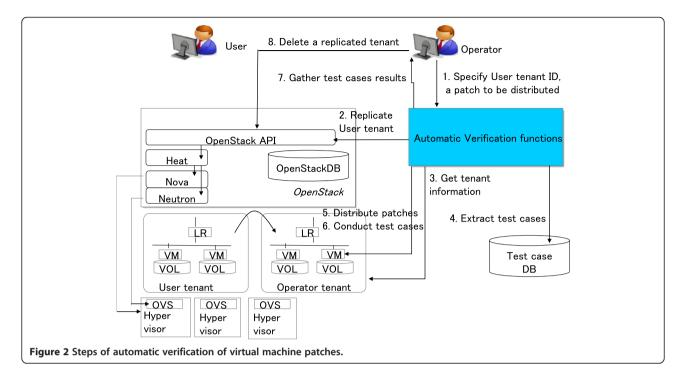
not only the GUI but also the API to start verifications. When verifications are handled for many users, a provider prepares a script program that extracts verification target users from a customer DB, manages released patches to be verified, schedules orders of each user tenant verification, and calls the AVF API to start verifications.
