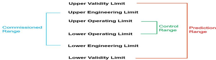
Figure 8.26 An illustration of variable limits [7]. Used with permission from Aspen Technology, Inc.
