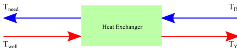
Figure 1: Generic Heat Exchanger Example. T_{well} is the temperature of the produced water at the wellhead; T_Y is the temperature of the water after the heat has been transferred to the secondary fluid and prior to being re-injected into the subsurface; T_{IN} is the temperature of the secondary working fluid prior to being heated from the produced water; T_{need} is temperature of the secondary working fluid after being heated from the produced water.
