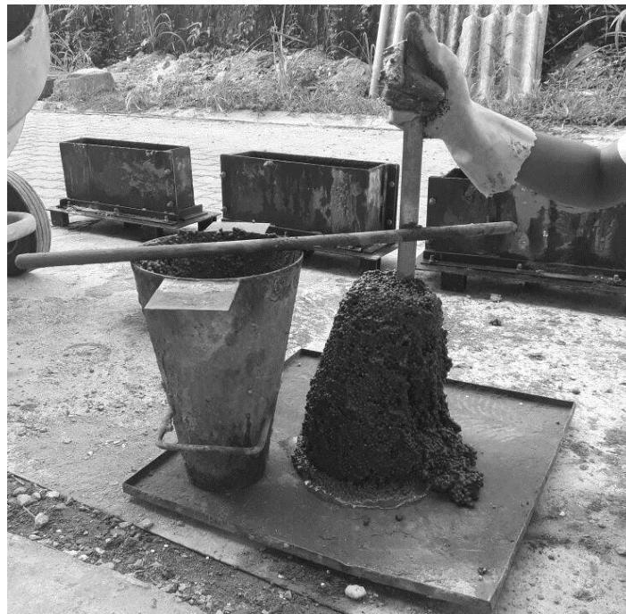
Figure 5 True slump of Mix 4
