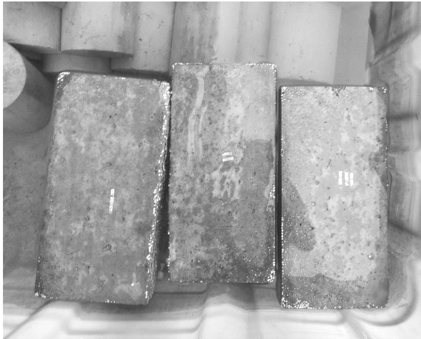
Figure 6 Blocks of Mix 4 floating on water
