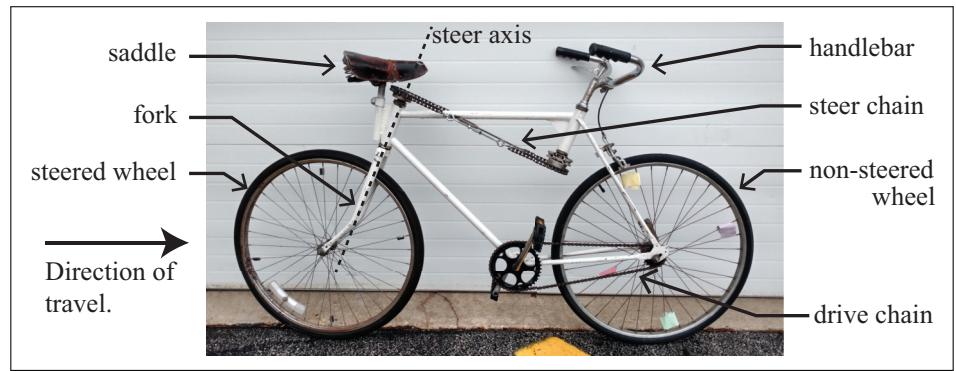
Fig 1. Klein’s “unridable bicycle.” A photograph of the rear-steered bicycle that Richard Klein and others deemed unridable.
