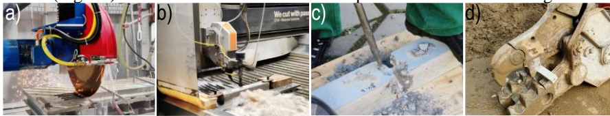
Fig. 2. Separation process by a) sawing, b) waterjet, c) hydraulic hammering and d) crushing.
