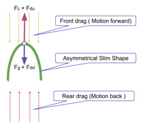
Fig. 1 Acting forces on asymmetrical slim shape
