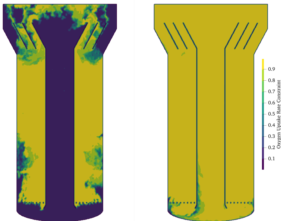
Figure 10: Mid plane contour plot of the oxygen uptake constraint from the spatial variability CFD model of the 300,000 litre ALR. Cell density from Li et al. [2020] on the left, from Negulescu et al. [2023] on the right
