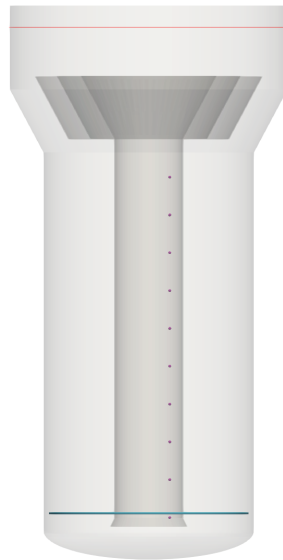
Figure 9: Schematic of the 300,000 litre airlift reactor with probe locations (purple), sparger (cyan) and media height (red line).
