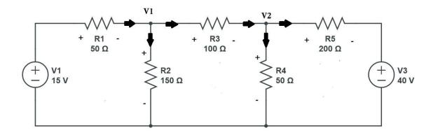
Let us label the flow of currents. We have two nodal voltages,  $V_1$  and  $V_2$ .
