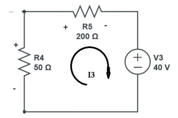
We assume the direction of current to be flowing in clockwise direction.
