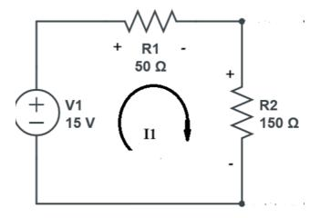
Current flows from lower potential to higher potential at  $V_1$  so it's polarity will be positive whereas current at  $V_{R1}$  and  $V_{R2}$  flows from higher potential to lower potential so its polarity will be negative.
