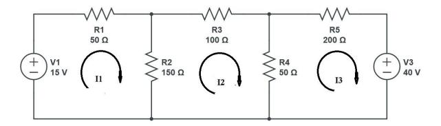
We have identified three loops, hence three loop currents I<sub>1</sub>, I<sub>2</sub> &I<sub>3</sub>.
