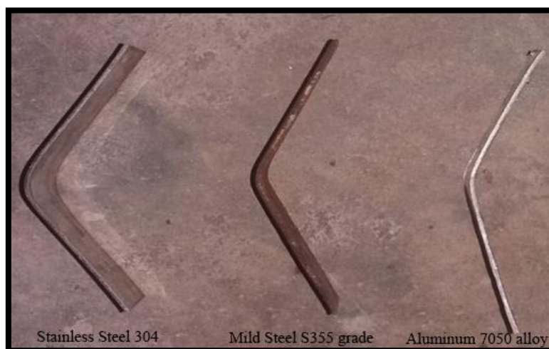
Fig. 4: deformed specimens of Stainless Steel 304, Mild Steel S355 grade, and Aluminum 7050 alloy.
