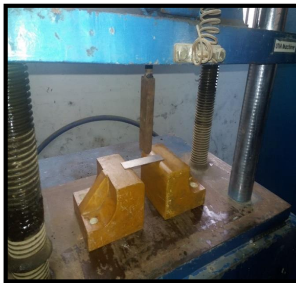
Fig. 2: A real view of experimental setup under a Universal Testing Machine for air-bending.
