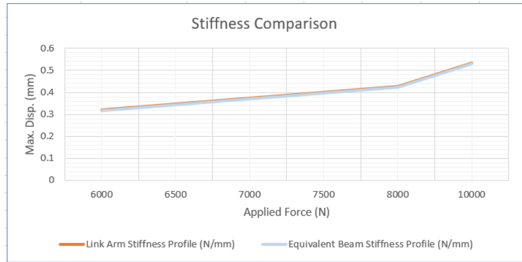
Figure 5. 15: Stiffness comparison between the link arm and the approximate beam.
