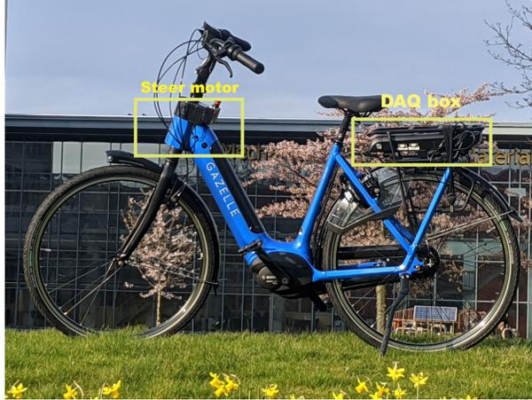
Figure 1: Balance assist bicycle prototype with electric motor in the steering column and data acquisition and control electronics mounted in the rear rack.
