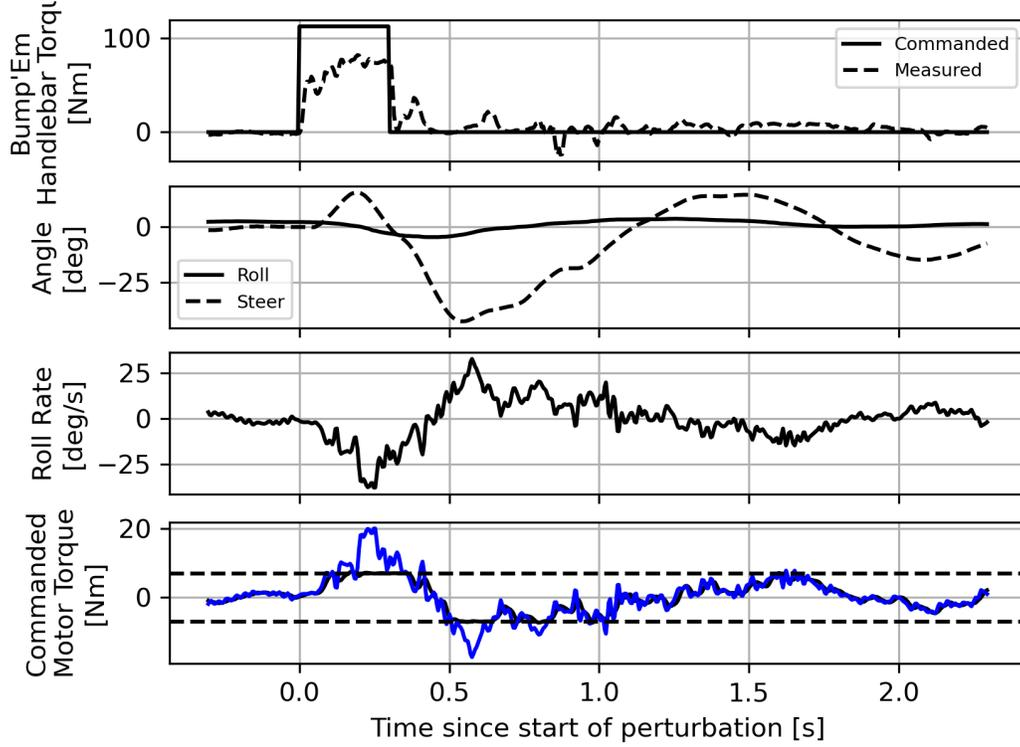
Figure 5: Motor force and resulting steer torque perturbation based on an 110N counterclockwise applied force.
