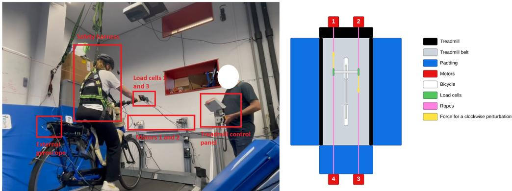
(a) A participant on the bicycle in the safety harness (b) Top view diagram of bicycle handlebar perturbation system with the Bump'Em motor lines attached to the ends of the handlebars.
