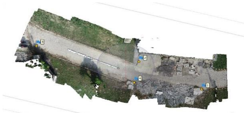
Figure 6: Dense point cloud before construction
