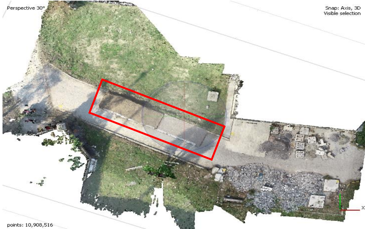
Figure 8: Dense point cloud post-application of aggregate base and subgrade layers, showcasing layer addition.
