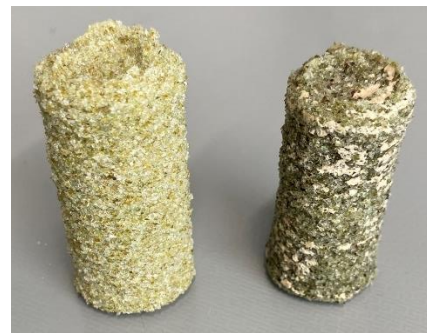
Figure 17. Glass samples. Left: As printed. Right: Reduced size after sintering.
