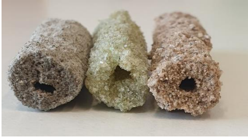
Figure 11. Hollow tubes were consistently formed in large single tracks bound with sodium silicate.
