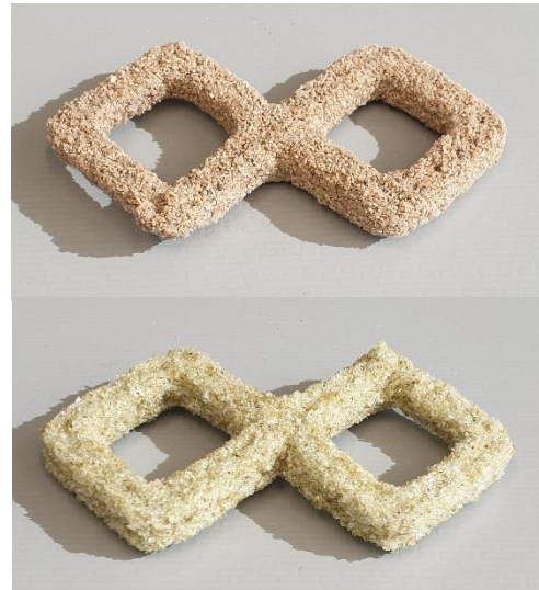
Figure 12. Custom diamond toolpath designed to test self-intersection of the toolpath printed with sand/PVA and glass/PVA.
