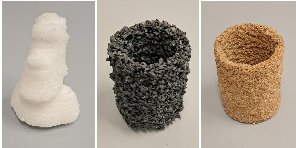
Figure 15. Left: Sugar/Sugar syrup moai. Middle: Granulated polystyrene waste/ABS-acetone cup. Right: Sawdust/Epoxy cup.
