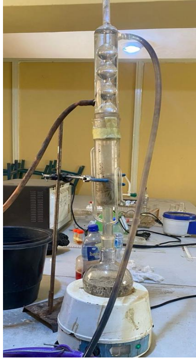
Figure 3.1: Soxhlet apparatus held by the retort stand and a measuring cylinder containing diesel
