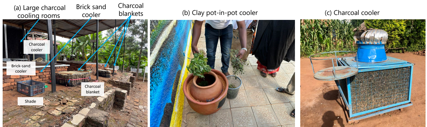
Figure 8. Different types of passive evaporative cooling devices. (credits: (a) Theresa Wittkamp in Kenya, (b) Eric Verploegen (amaranth after 1 day stored in a clay pot cooler (left) and in a plastic basket (right) in Niamey, Nigeria, by CoolVeg ( https://www.coolveg.org/clay-pot-coolers )), (c) Charcoal cooler to store fruit and vegetables at a smallholder farm in rural Uganda (photo credit: Jakub Vrba).
