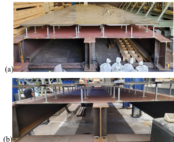
Figure 5: 12.2m x 3.0m (40’ x 10’) vibration specimens (a) W24x68 with 9.5mm (3/8 in.) PL. and RAF (b) W24x94 with 12.7mm (1/2 in.) PL. and RAF
