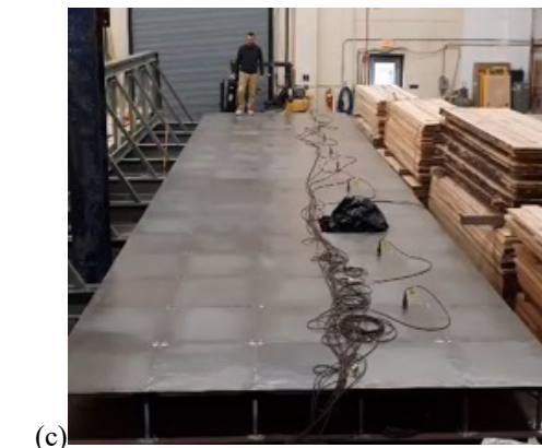
Figure 6: Example excitations on vibration specimens (a) impact hammer (b) shaker (c) walking
