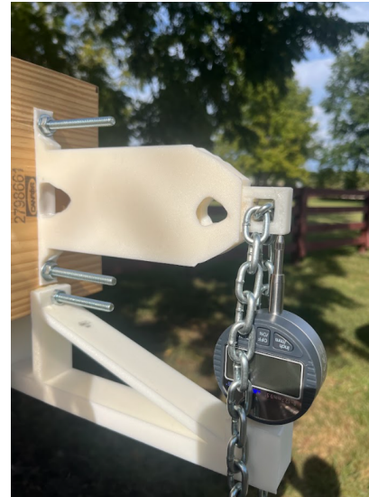
Fig. 19: Experimental setup for testing displacement
