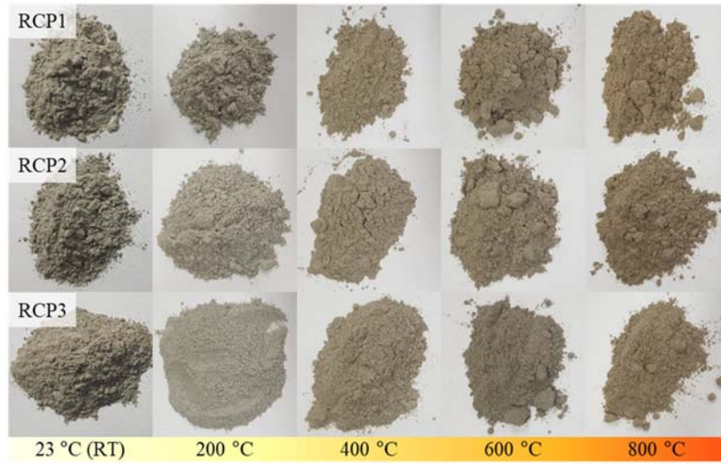
Figure 2. Multi-recycled concrete powders before and after heat treatment
