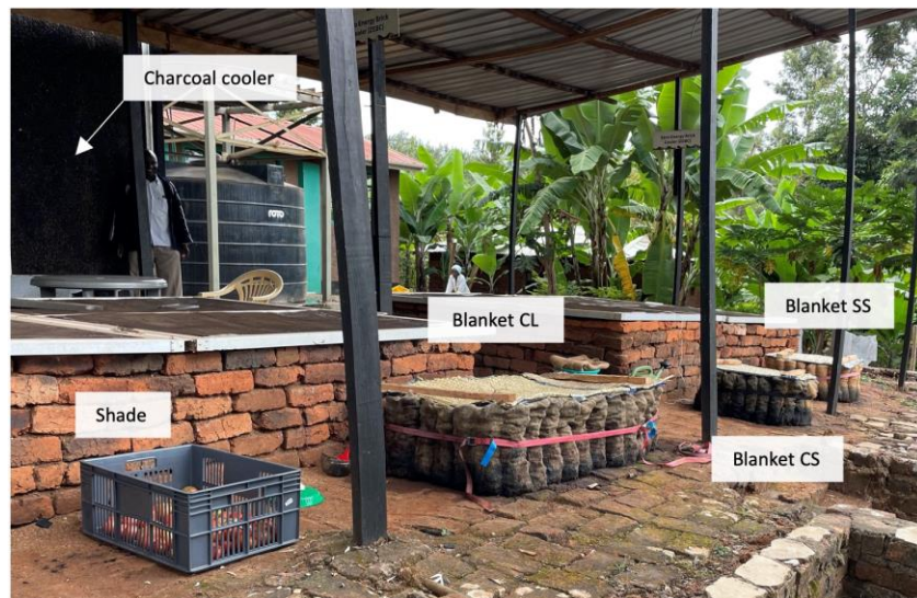
Figure 1: Overview of the different cooling systems at the study location. Three cooling blankets were tested simultaneously (CL = charcoal large, CS = charcoal small, SS = sawdust small) and compared with storage in a large charcoal cooler and shade.
