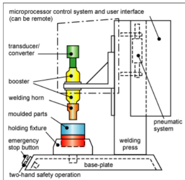
*Figure 4: Schematic of ultrasonic welding machine*
