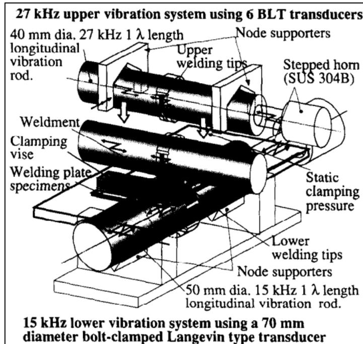
*Figure 9: The ultrasonic lapped spot-welding system uses two longitudinal vibration sources with 27 kHz and 15 kHz systems, arranged at a right angle*
