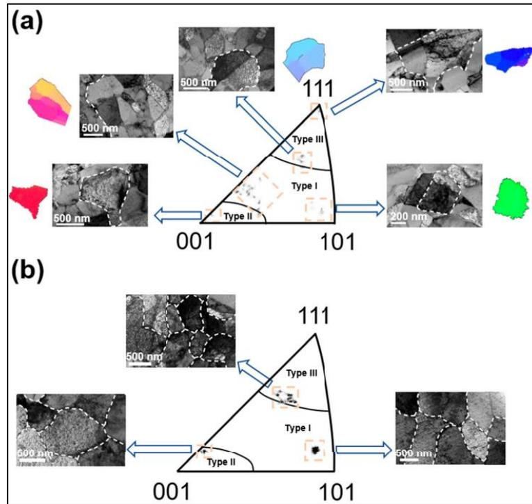
**Figure 14:** TEM images and orientations of target grains in (a) DRX grains and (b) shear-deformation regions, divided into Type I-III per Hansen and Winther's research
