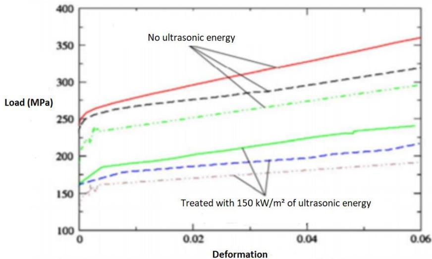
**Figure 13:** Effect of ultrasound on tension
