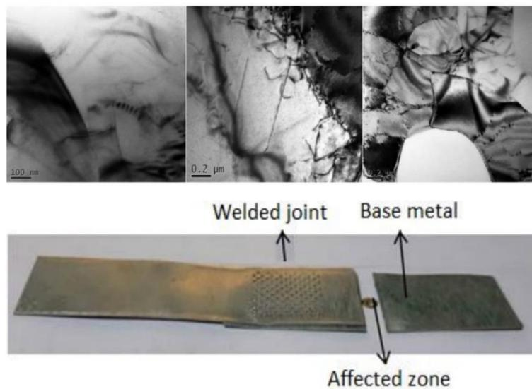
*Figure 17: Welded aluminum foils and TEM images of base metal*
