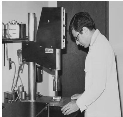
*Figure 3: Robert Soloff with ultrasonic welding press 1960s*
