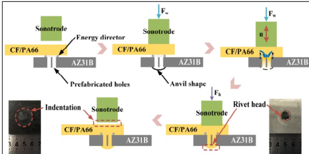
**Figure 7:** Schematic diagram of the ultrasonic extruded weld-riveting process. “ $F_w$ ” means the welding force; “ $F_h$ ” means the holding force
