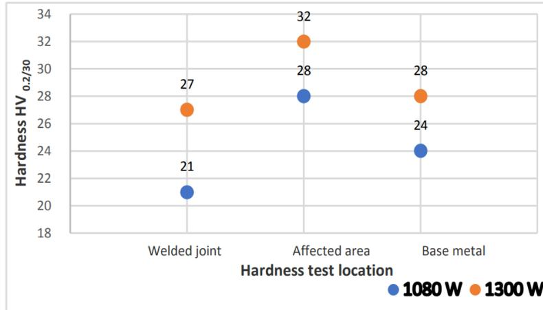
**Figure 19:** Microhardness test values depending on the distance of the welded joint
