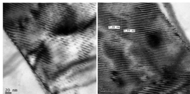
*Figure 18: TEM image of welded zone*
