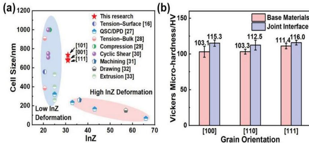
**Figure 15:** (a) Shows the relationship between  $\ln Z$  and dislocation cell sizes in pure copper, using parameters from various studies. (b) Displays Vickers microhardness comparisons between the base materials and the joint interface, showing stronger hardness at the joint.
