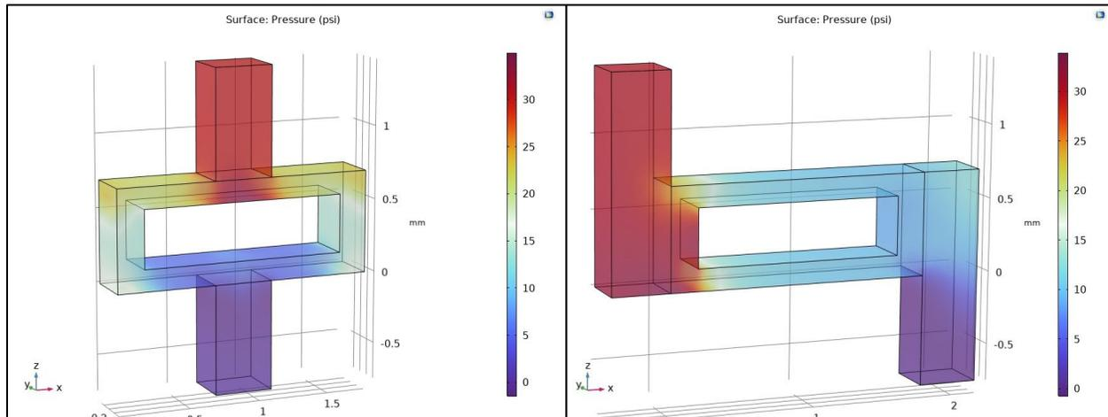
**Figure 2 COMSOL CFD Simulation showing the pressure distribution on the membrane for the “Perpendicular Control” Valve.** Left: Pressure distribution on the membrane of the naive design under actuation, highlighting unevenly high stresses at the membrane center, potentially leading to rupture or mechanical failure. Right: Pressure distribution on an optimized design, demonstrating how stresses are shifted away from the membrane’s center—the weakest part—toward more structurally robust regions.
