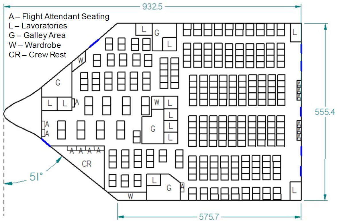
Figure SI 3. Cabin layout of NASA N+2 BWB aircraft for 301 passengers where dimensions are in inches (source [10], Copyright: work of the US government and public use is permitted)
