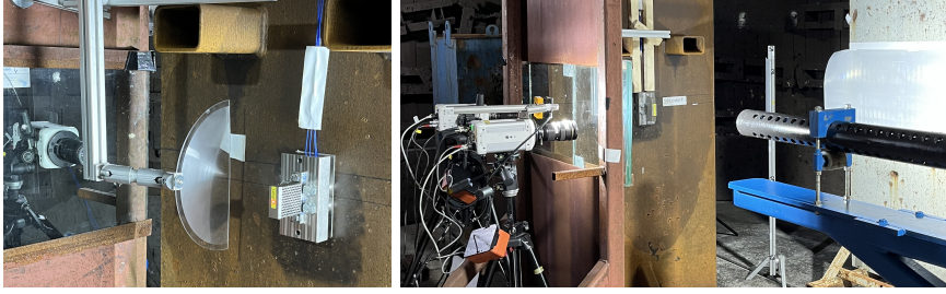
(a) Position of the camera with Fresnel lens. (b) Shooting barrel and camera pointing at the sample.
