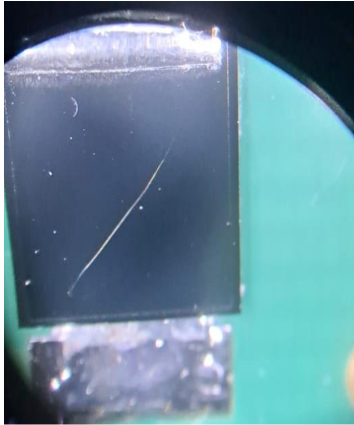
Figure 7. Example of failed visual inspection
