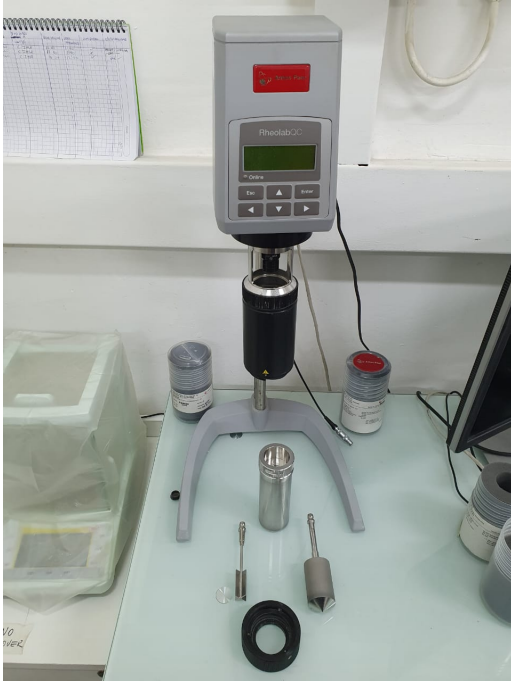
(a) Typical installation of a concentric cylinder rheometer
