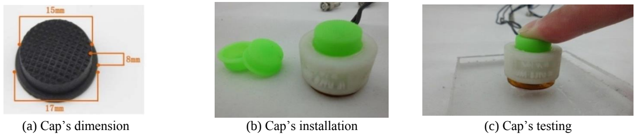
Fig. 6 Cap's dimensions and the final assembled prototype
