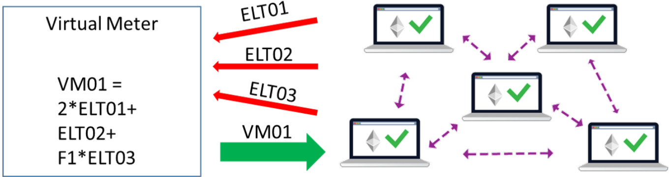
Fig. 18: The consumption of Virtual Meters gets calculated from the consumption of their associated Smart Meters.
