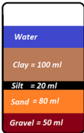
Fig. 3. Granulometric jar test.
