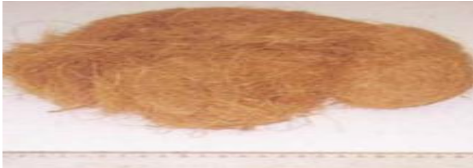
Fig 2: Extracted Coconut Coir Fibres
