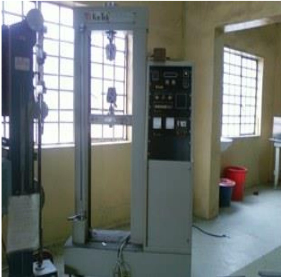
Fig 2.6: Universal Testing Machine - UTM (Kao Tieh testing machine) for Tensile Testing
