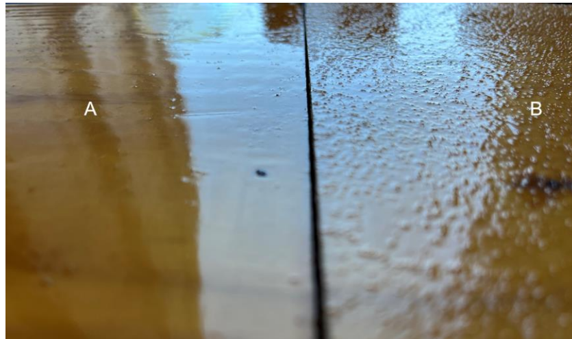
Figure 2. A photograph exhibiting the difference between a wood piece with 2 coats of stain and sealer with no sand additive (A) compared to a wood piece with sand additive mixed into the first coat and covered with a 2 nd coat of stain and sealer (B).
