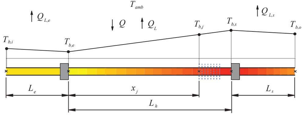
Figure 5: Temperature variation along the test section.
