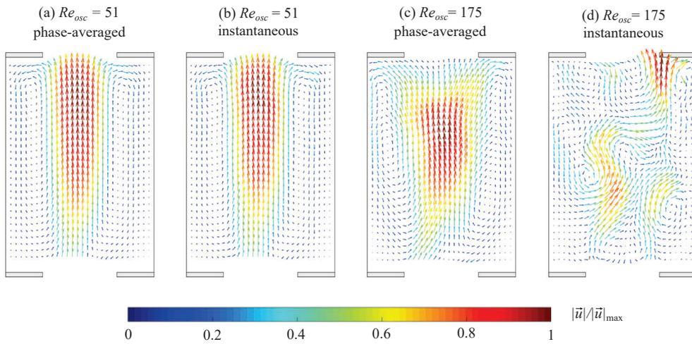
Figure 9: Phase-average vs. instantaneous velocity fields. Pure oscillatory flow
