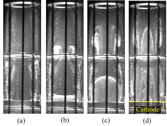
Figure 7: Front view of the hydrogen bubble seeded plane for  $Re_{osc} = 32$ . (a)  $\theta = -22^{\circ}$ , (b)  $\theta = 22^{\circ}$ , (c)  $\theta = 55^{\circ}$  y (d)  $\theta = 90^{\circ}$ .  $x_0/D = 0.5$ .
