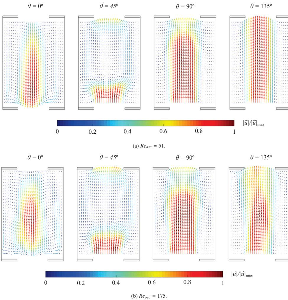
Figure 10: Phase-average velocity field for different instants of the oscillation cycle. Pure oscillatory flow.
