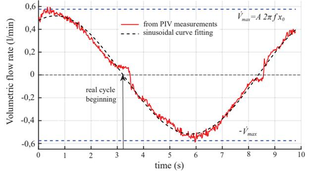
Figure 3: Instantaneous volumetric flow rate obtained from the PIV velocity field.
