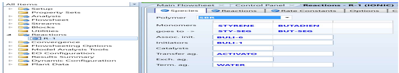
Figure 6.61 Species specification of the ionic reaction set R-1 for anionic copolymerization of styrene and butadiene.
