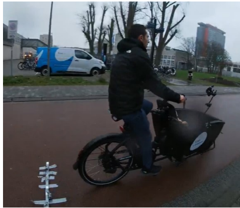
Figure 21: We performed a shock test with bicycles riding over a 30x30 mm square section bar. ALT TEXT: Photo of cargo bicycle shock test.
