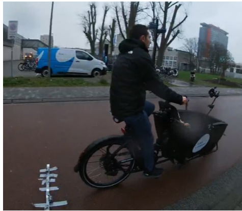
Figure 32: We performed a shock test with bicycles riding over a 30x30 mm square section bar.
