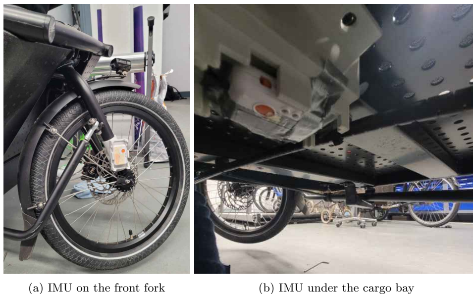
Figure 23: IMU locations on the Urban Arrow. The white 3D printed sensor supports are visible in (a) and (c). The last figure (d) shows how the sensors were taped to the seat pan and backrest.
