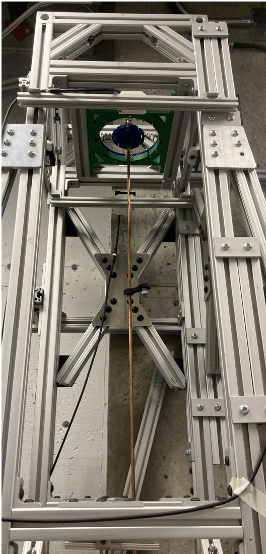
Fig. 2 A photograph of the VARM built and tested at Polytechnique Montréal. For reference, the shaft length from the upper bearing to the lower bearing is 850 mm.
