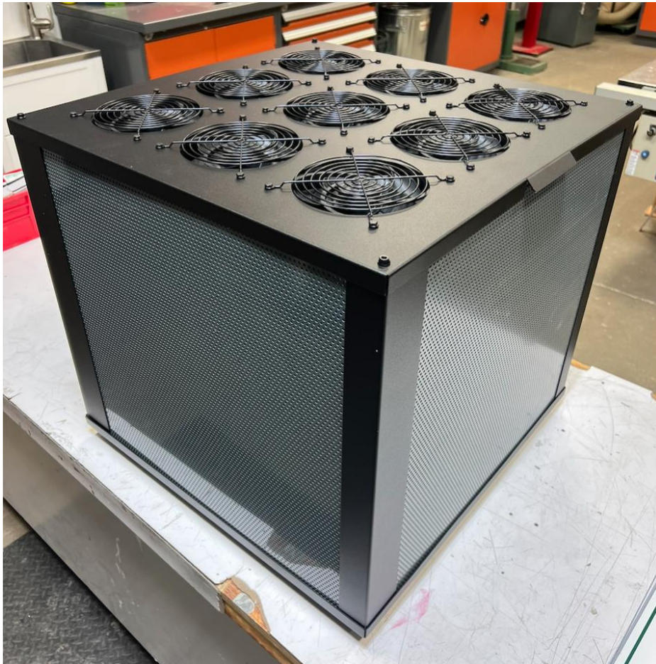
Image 2: Nine Fan, Four Filter DeisBox with Predicted CADR >500CFM (TBD)
