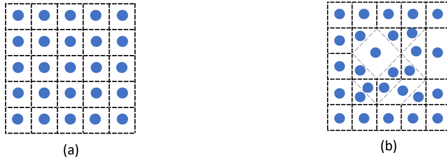
Fig. 2. Element centroids for (a) a uniform part of the mesh and (b) a non-uniform part of the mesh are chosen as PD nodes. The element area is used as the PD nodal area.
