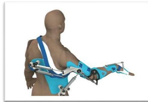
Image 6 - A three-bar linkage system illustrating elbow articulation
