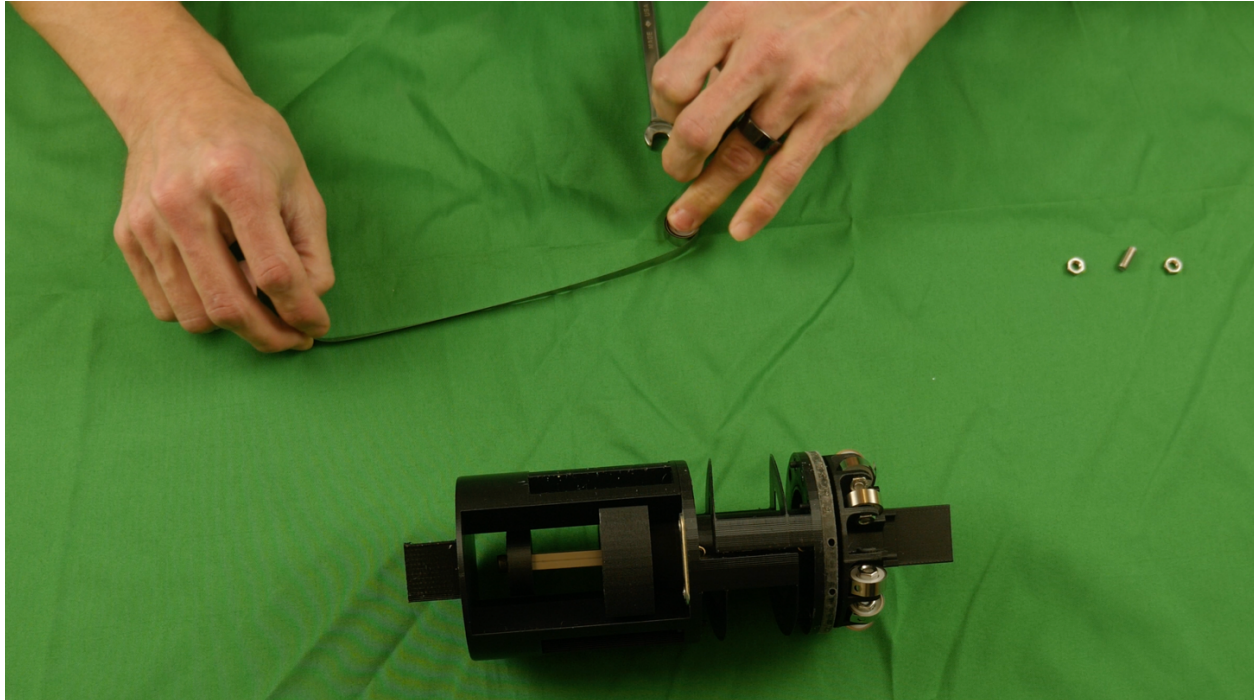
Fig. S2. Constant-Force Spring Assembly. This photograph demonstrates extension of the c-f spring and seating of its inner ring on the outside of a ball bearing. The bolt and nuts used to attach the c-f spring to the grounded body are shown at right.
