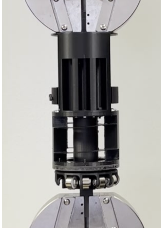
Fig. 4. Universal machine testing setup for force profile collection. We mounted the bearing vertically between two wedge action grips to measure the quasi-static force throughout its full range. For a time-lapse of a test of the bearing with each of the retention mechanisms, see supplementary Movie S2.
