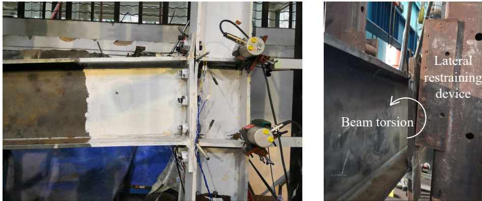
Figure 5. Failure mode of Specimen B355-C690-EP16-WCF
