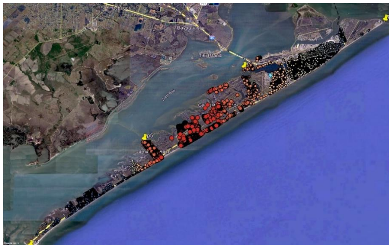
Figure 12. Focused distribution of DS3 damage state in Galveston under Scenario Hurricane HR1.
