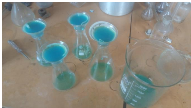
Figure 45: filtering the leachate solution
