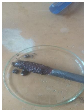
Figure 46 : recovery of copper from PCB & metal powder by electrolysis
