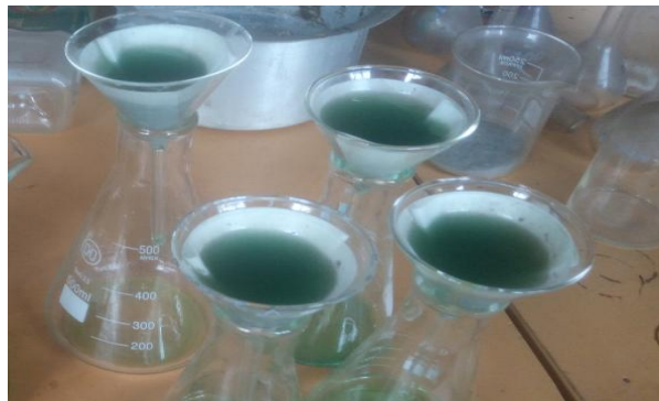
Figure 45: filtering the leachate solution
