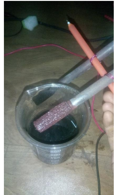
Figure 37: recovery of copper from PCB & metal powder by electrolysis
