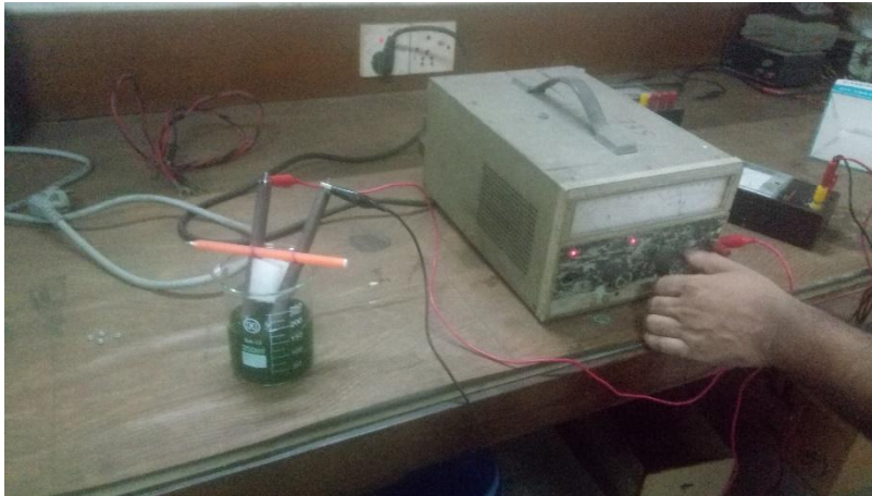
Figure 37: recovery of copper from PCB & metal powder by electrolysis
