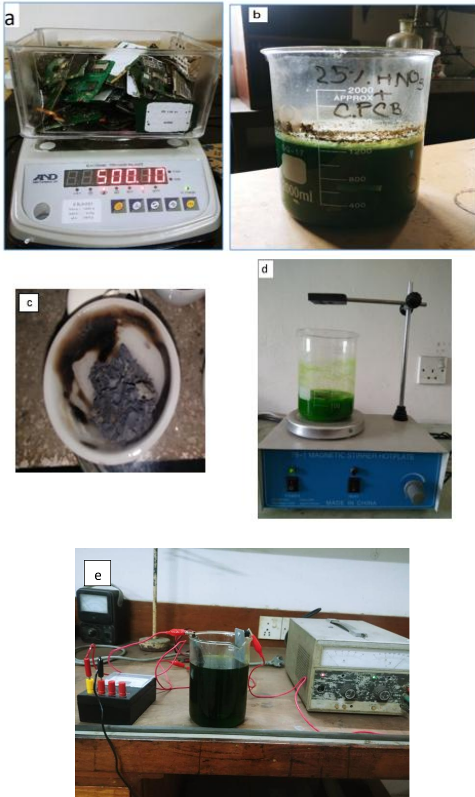
Figure 51: Figure 4. Different stages of Tin extraction: (a) Sample preparing (b) Acid Dissolving (c) Burning at 600C (d) Leach liquor stirring in HCl and Zn (e) Electrodeposition process
