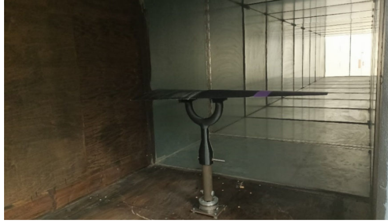
Figure 7. The model test section of inside the wind tunnel.
