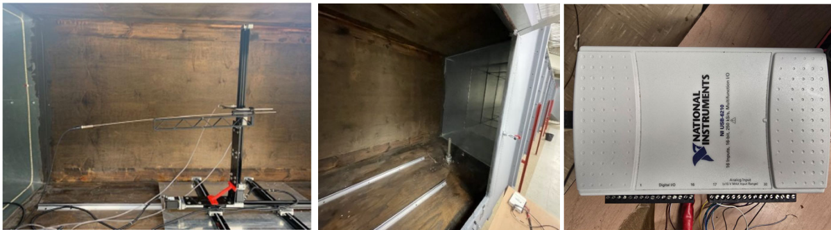
Figure 13. (a) Traverse system, (b) load cell boom arm, and (c) DAQ
