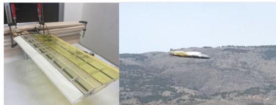
Figure 08. (a) RSAWC wing with covering, and (b) UAV with RSAWC wing during flight test [38]
