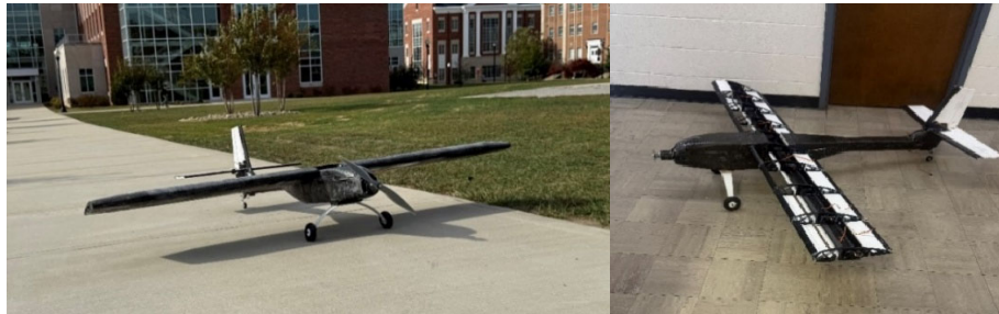
Fig. 21 (a) Complete assembled and (b) without wing skin
