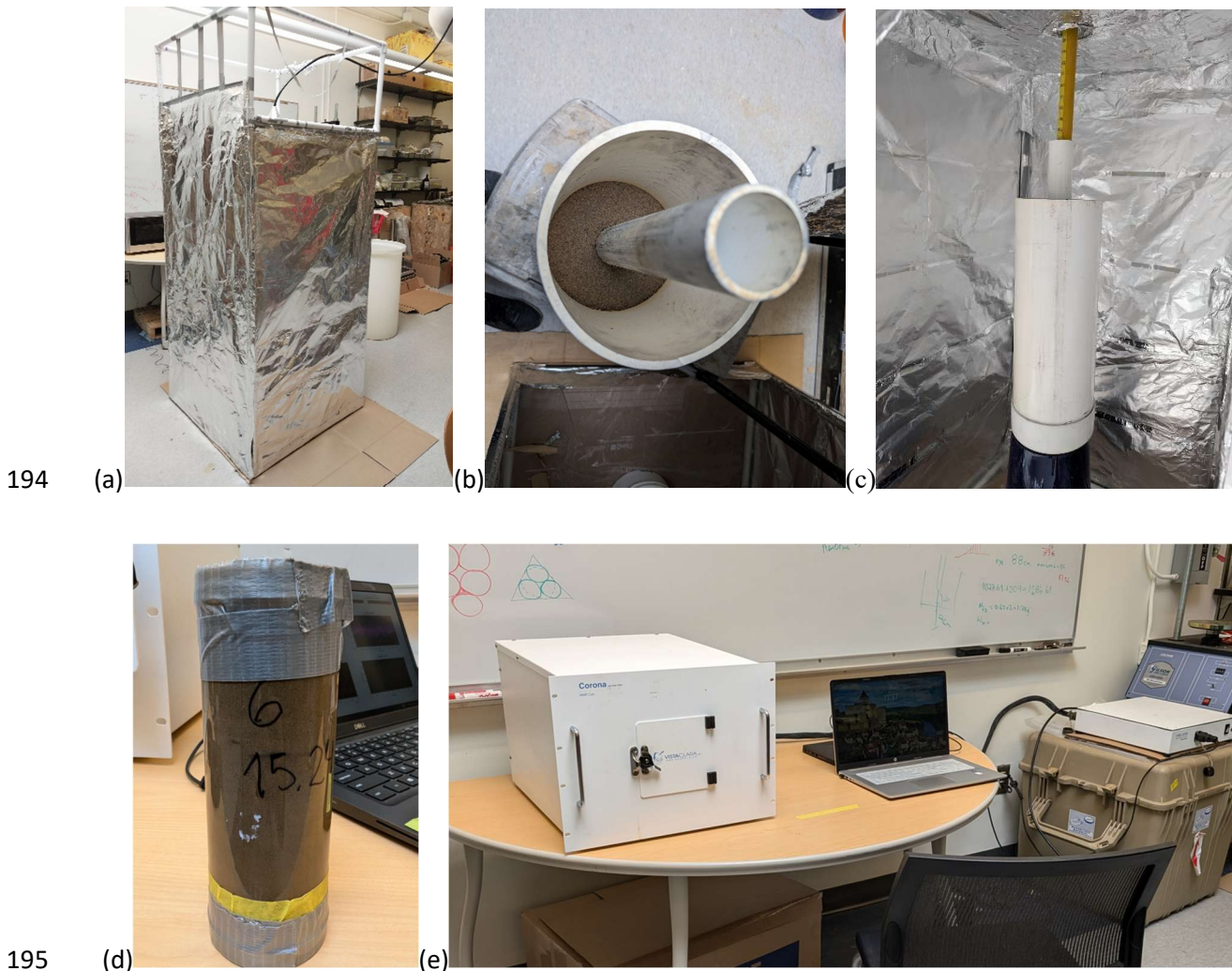
196 Figure 5. (a) Faraday Cage enabled for NMR Dart measurements, (b) top view of the PVC container with 197 mine tailings being placed, (c) example of the Dart probe inside de Faraday cage during an NMR 198 measurement, (d) container used for Helios measurements, and (e) set up during NMR measurements in 199 the Helios chamber.
