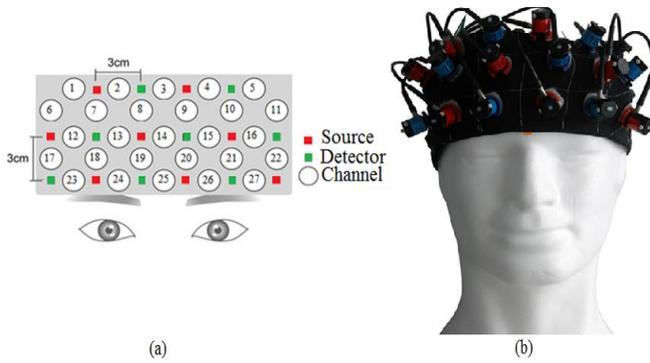
**Figure 2.** Measurement setup: (a) channel configuration and (b) probe holder worn on the PFC area. Eight sources and eight detectors used in the measurements corresponding to 27-channels over the PFC area.
