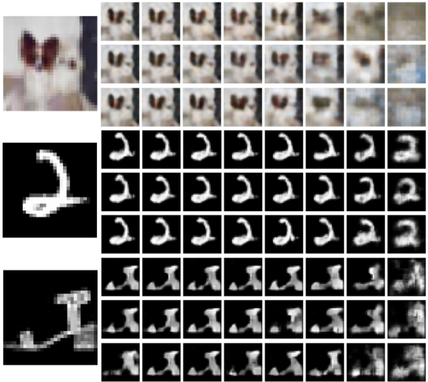
Figure 1.5: Visual comparison of model inversion attack reconstructions for CIFAR10, MNIST, and FashionMNIST datasets across baseline, DP_{\epsilon=2} , and L2+Dropout model configurations, showing reconstructions from each network layer [1].
